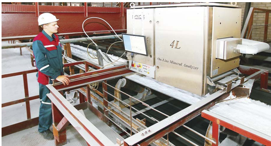
Figure 4. Lyncis online element analyser in operation at Belaruskali facility.
